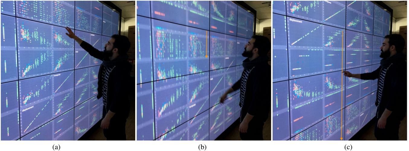
**Figure 7:** A continuous vertical paternoster is triggered by a three-finger-fling downwards (a). The matrix is moving at a constant speed in (b) until it is stopped by a tap in the desired location (c). The orange arrow shows the already traveled distance in (b) and (c) respectively. Due to the cyclic scrolling of the matrix the rows that were pushed out at the bottom of the display re-appear at the top.
