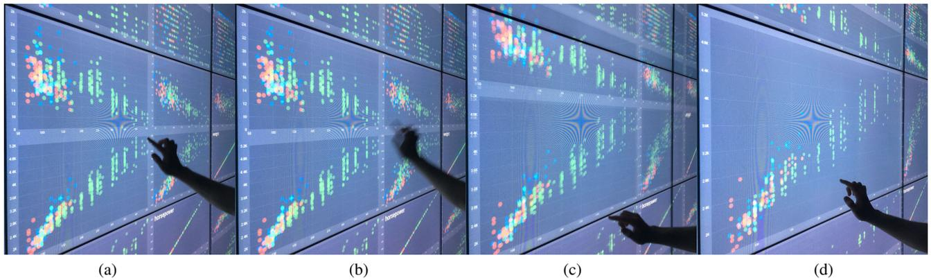
**Figure 3:** Global F+C by resizing a plot with a fling gesture. A fling is applied on the corner (subfigure a and b). The plot expands with a constant speed (subfigure c) until it is stopped by a single tap (subfigure d). The matrix-wide effects can be seen in Figure 5.
