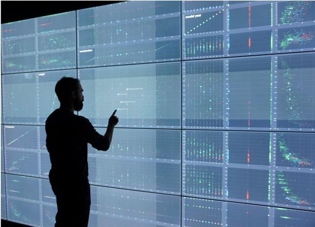
**Figure 1:** Touch-enabled visual analysis using SPLOMs on a large wall display ( $4.08 \times 2.31$  m). Our two-tiered Focus and Context (F+C) technique with an outer F+C at matrix level and an inner F+C within scatterplots improves the exploration process by giving access to detail even in dense areas (see Subsection 3.1).
